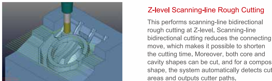
Z-level Scanning-Line Rough Cutting This performs scanning-line bidirectional rough cutting at Z-level. Scanning-line bidirectional cutting reduces the connecting move, which makes it possible to shorten the cutting time. Moreover, both core and cavity shapes can be cut, and for a composite shape, the system automatically detects cutting areas and outputs cutter paths.
