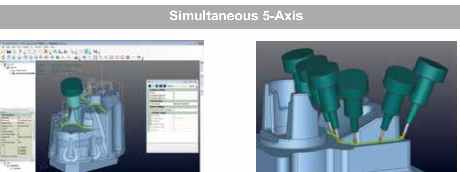
Simultaneous 5-Axis 5-Axis conversion function Creates 5-axis Simultaneous tool paths, by adding the information about tool direction to 3-axis tool paths. In converting tool paths, "smoothing control" adjusts the tilt axis and rotation axis to make the Machine Tool move more smoothly. It is also possible to have the tool tilt gradually before the point where the tool direction changes rapidly. These functions provide high-quality finished surfaces. Automatic interference avoidance Collision of Tool, Chuck and Holder with the shape can be avoided by controlling tilting axis automatically. Change tool direction gradually to avoid drastic change of tool direction. It minimizes the cutting mark.
