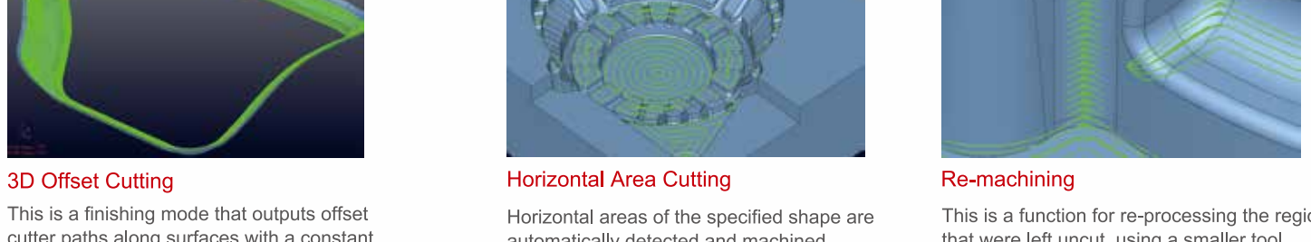
Horizontal Area Cutting Horizontal areas of the specified shape are automatically detected and machined. The climbing cut is always performed and cutter paths traveling around (contour line) are output. The output NC data consists of G01 with simultaneous two axes (Simultaneous three axes for slant cutting). This mode is useful for the shape, containing many horizontal areas and requiring bottom machining with a flatnose tool. Re-machining This is a function for re-processing the regions that were left uncut, using a smaller tool. Based on the radius of the previous tool, remainder regions are automatically detected and cutter paths are generated for those regions only. Cutting of remainder regions can be performed along ridgelines or perpendicularly to ridgelines, depending on the angle of the ridgeline.
