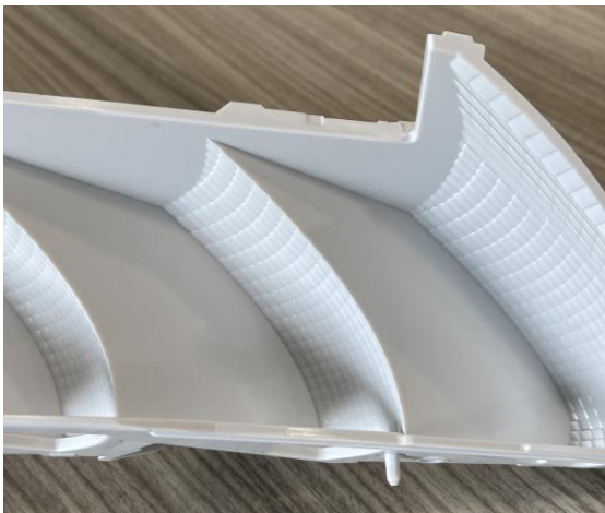
An example of a Reflector that requires “Ra: 1.5 \mu -2 \mu ” of mold surface accuracy without polishing
